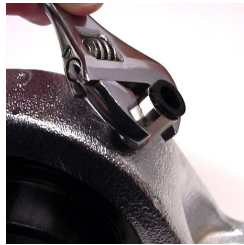
5. Install the tubing fitting on bearing or lube point.
