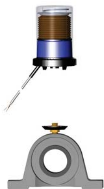
Program the MEMO fitting and install it on the lube point.
