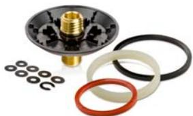
The MEMOLUB® EPS daily lubricant output is programmed using the simple MEMO system. The Red, White and Black timing rings determine how often the lubricator will cycle. The seven basic time settings required to handle most applications are programmed by using one, two or all three colored timing rings. To fine tune the lubricant output, you can adjust the piston stroke by installing the spacer washers into the MEMO
