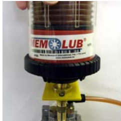
8. Screw the MEMOLUB® lubricator onto the MEMO fitting. Your MPS System is ready to go!
