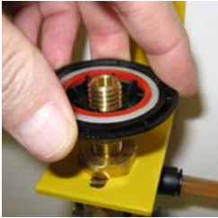
4. Gently press the black timing ring holder onto the MEMO fitting.
