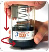
1 To open, place the lubricator upright on a flat surface. Press down firmly on the clear housing and turn the locking ring counter-clockwise while holding the ribbed surface.
