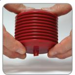
4a Carefully squeeze any air out of the cartridge until grease begins to emerge from the outlet.
