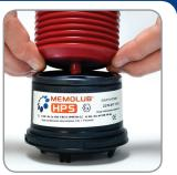
4b Place the lubricant cartridge on the inlet of the pump housing.
