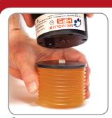
Sa Carefully remove the plug. Place the battery seal onto the cartridge. Turn the pump over and gently place it on the outlet of the cartridge.
