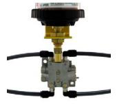
Using a MEMOLUB<sup>®</sup> distribution block, the MEMOLUB<sup>®</sup> HPS Multi-Point System can service from 2 to 12 lubrication points. The distribution block is completely sealed to keep out airborne contaminants, dust, and dirt, and works on the principal of piston valves. During operation, a series of pistons inside the block is actuated by the flow of lubricant from the MEMOLUB<sup>®</sup> lubricator. Lubricant flows through a
