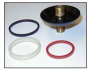
The white, red, and black plastic timing rings are used to set the frequency of ejection cycles of the MEMOLUB<sup>®</sup> HPS. They are inserted into the black plastic ring-holder either individually or in combination to obtain the desired frequency of output cycles.
