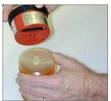
the red housing, reverse their position. Place the red housing and cartridge on a hard surface and place transparent housing on top. Lock as instructed in *Section 6.2.2*.
