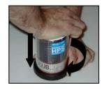
To close, use the same technique. Pressing down on the housing, hold the locking ring by its ribbed surface and turn it clockwise until it clicks into the locked position. Ensure that the locking ring locks by holding the ring on its smooth surfaces and turning clockwise. If the housing is correctly locked into place, it will not be possible to open it while holding the locking ring on its smooth surfaces.
