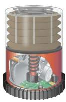
The lubricator body consists of a red motor housing, a transparent dome, a spring, a compression plate, a black rubber seal, and a black locking ring. The red motor housing contains all of the electromechanical parts of the MEMOLUB<sup>®</sup> HPS. The black rubber seal covers the battery compartment. Because of the configuration of its grease cartridge, the Model 480 lubricator does not require this black seal.
