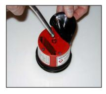
• Lift the black rubber seal back to reveal the battery chamber, and insert the battery pack into the red housing by holding it by its strip. The battery pack has to be inserted according to the instructions on the red housing. When the battery pack is inserted, the motor will be activated for a second. Put the rubber seal back in place. {*Note: The black rubber seal is not used on the Model 480, Giga lubricator.*}
