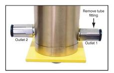
**Step 1.** Remove MEMOLUB® HPS lubricator from Spliiter-MEMO Remove push-in tube fitting from outlet No. 1. Screw in Zerk grease fitting supplied with Splitter-MEMO.
