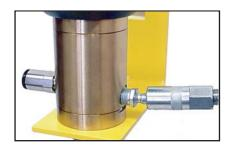
**Step 2.** With a standard grease gun inject grease through the Splitter-MEMO until grease comes out the top.
