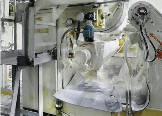
MEMOLUB MPS-2s lubricate roller bearings on paper coating equipment at Appvion paper plant.
