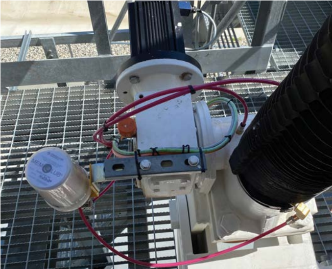
3-point system lubricating elevation jackscrew assembly on General Dynamics antenna.
